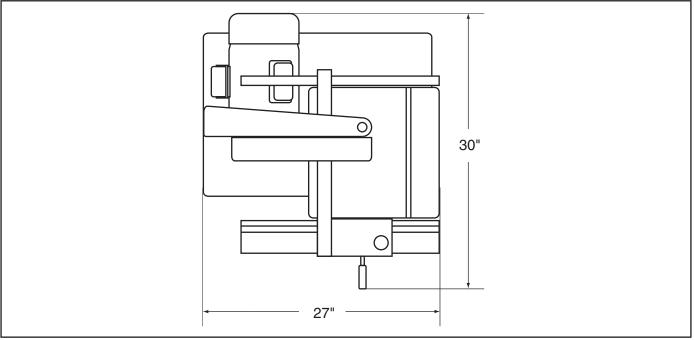
Figure 7. Minimum working clearances.
